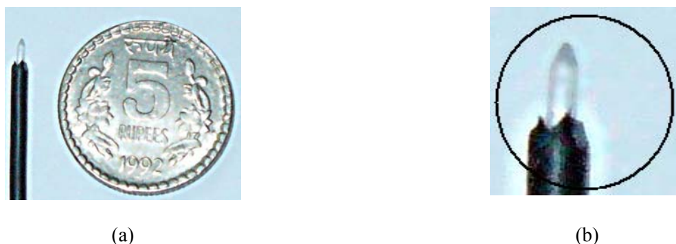
Fig. 1. (a) Photograph of an angled-tip optical fiber; (b) Magnified view of photo (a). For dimensional comparison a 5 rupees coin is also shown in the photograph. The angle of the fiber tip was measured to be 50^\circ .
