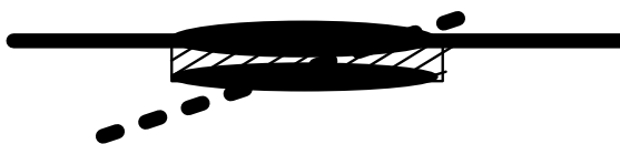
Fig. 3. Single node of the sensor: Two nodes are put together with insulating cement (expressed as shadow).
