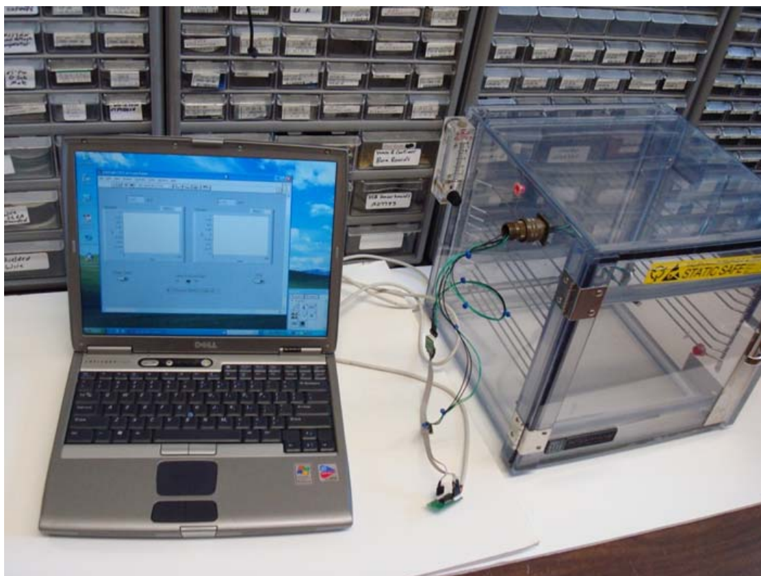
Fig. 3. Test chamber with LabView interface to laptop computer.
