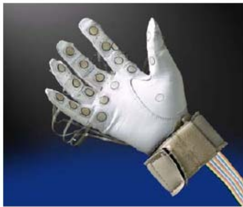
Fig. 7. Sensor placement on the force glove.
