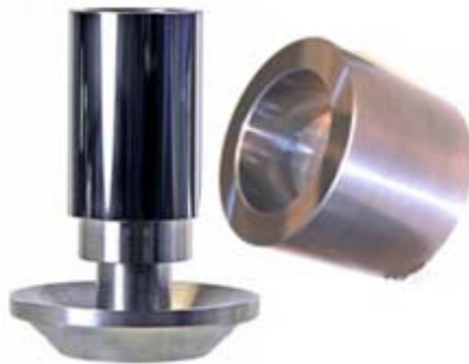
Fig. 2. Photographic view of the PC-NIS1 (Piston on the left and cylinder on the right).
