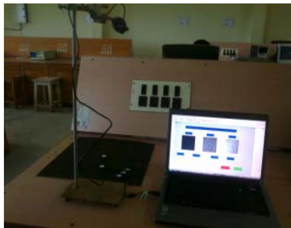
Fig. 14. Experimental setup for angular orientation measurement of robotic arm.
