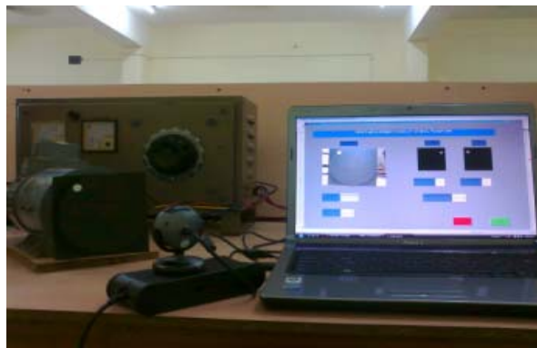
Fig. 11. Experimental setup for angular speed measurement.
