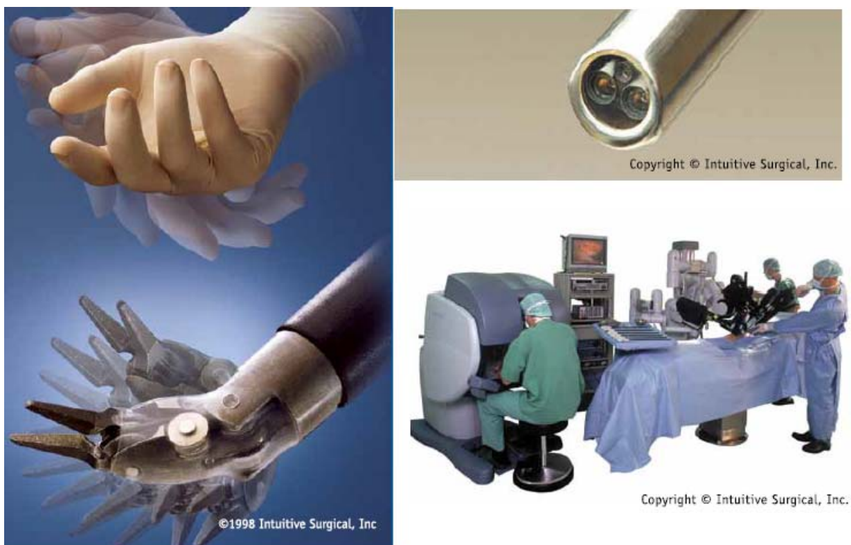
Fig. 1. MEMS based Intuitive Surgical da Vinci Robot [2].
