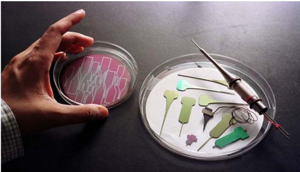
Fig. 2. MEMS based micro machine cutting tools [3].
