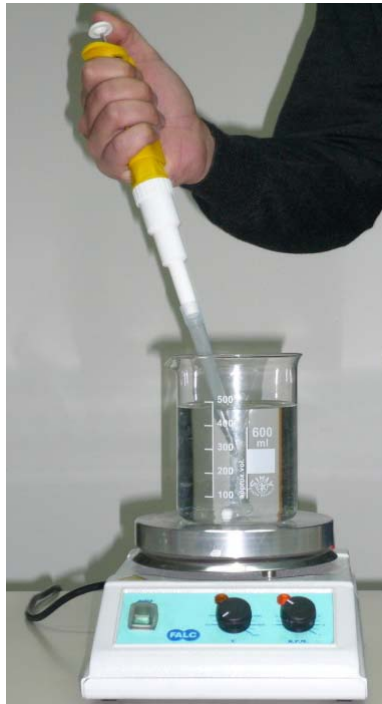
Fig. 1. Sample solution withdrawal from a continuously stirred beaker.
