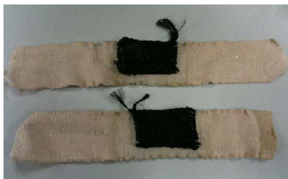
Fig. 3. Woven polypyrrole ECG pads.
