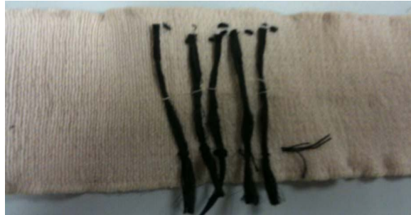
Fig. 2. Test structure to determine the basic contact resistance of the polypyrrole to the researchers skin.
