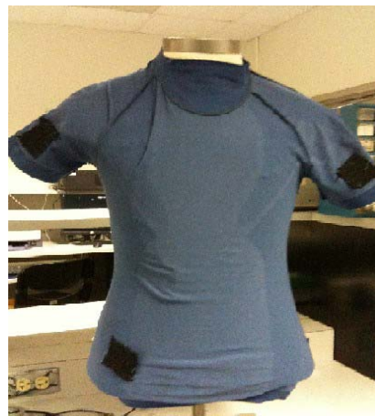
Fig. 4. Construction of the electrode assembly (T-shirt inside out).
