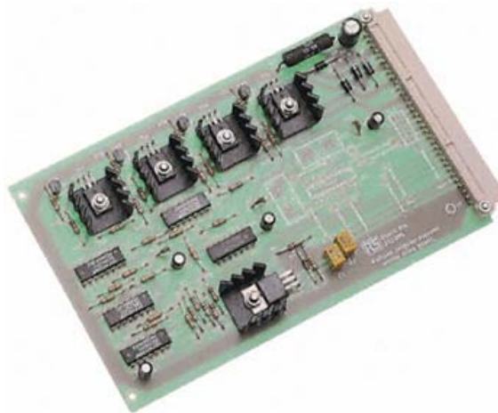
Fig. 9. The driver board used to run the motor [3].
