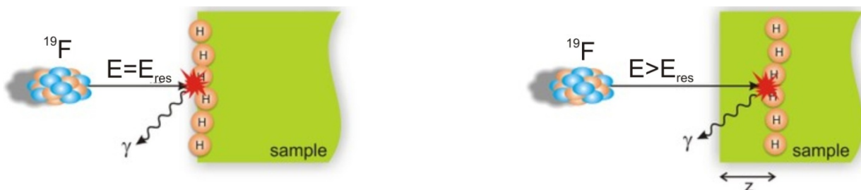
Fig. 6. Hydrogen depth profiling principle using (^{19}\text{F}, \alpha\gamma)^{16}\text{O} nuclear reaction.
