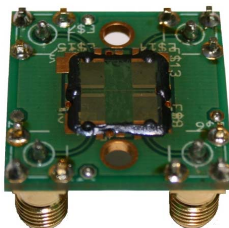
Fig. 2. Photograph of the SAW device using Love waves at 125 MHz.
