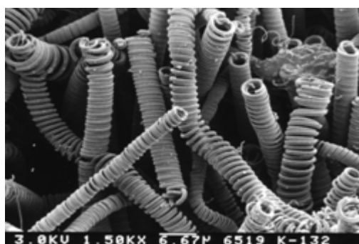
Fig. 1. Representative SEM image of double-helix carbon microcoils (DH-CMCs).
