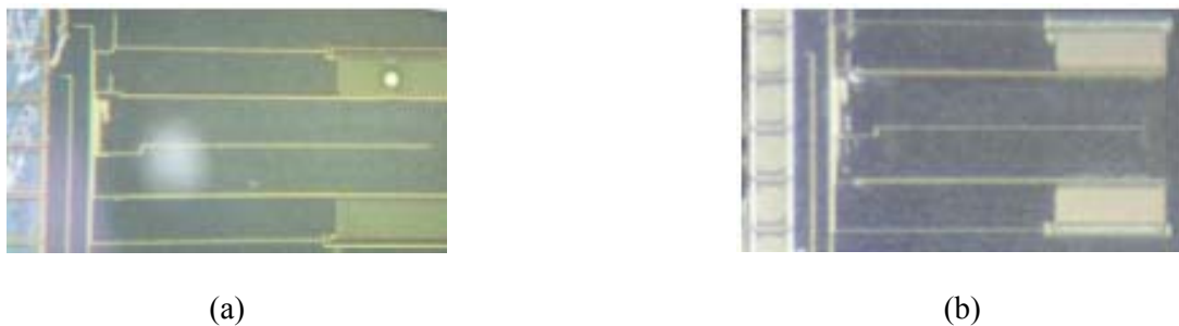
Fig. 5. Color change during Anisotropic RIE of SiO 2 (a) golden color of the sensor surface before RIE; (b) white color of the sensor surface after RIE.
