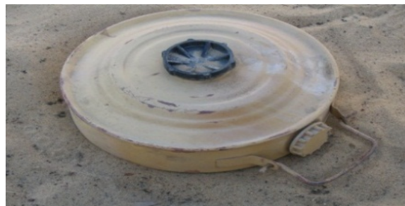
Fig. 5. T-71 Anti-Tank Landmine used in the experiment.
