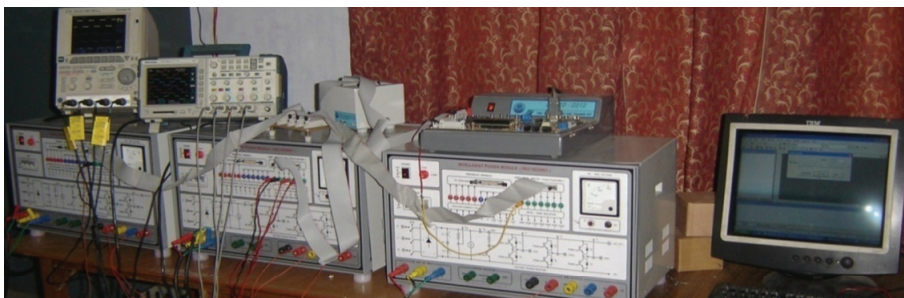
Fig. 12. The quasi-six phase voltage source inverter set-up.
