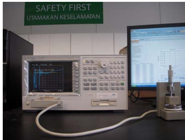
Fig. 2. Equipment used for measuring the permittivity and the conductivity of meat, which consists of Agilent 4294 impedance analyzer connected with Agilent 16451B dielectric fixture.
