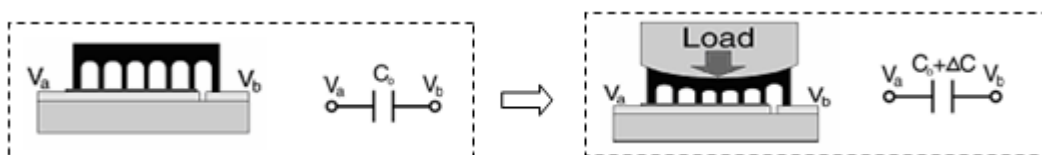
Fig. 3.7. Schematic of the Collapsible Capacitive Sensor Operation.
