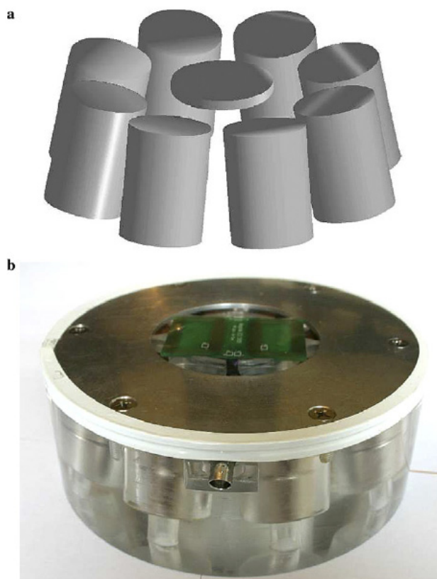
Fig. 6. (a) The configuration of magnets used to produce a homogenous region [5, 8]. (b) The complete prototype NMR-MOLE probe. The magnets are placed into a plastic housing and the B_1 coil is placed onto the surface as shown.
