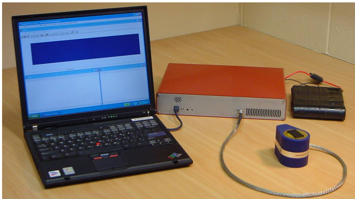
Fig. 13. Complete battery powered portable NMR system. The spectrometer part measures 310x230x55 mm and weighs 3.6 kg. The battery pack shown can provide 3 to 4 hours of operation, depending on the RF power requirements.
