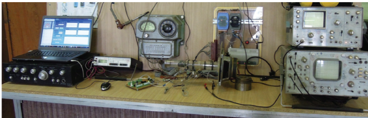
Fig. 7. Experimental plant for standing wave thermoacoustic refrigerator overall efficiency calculation.
