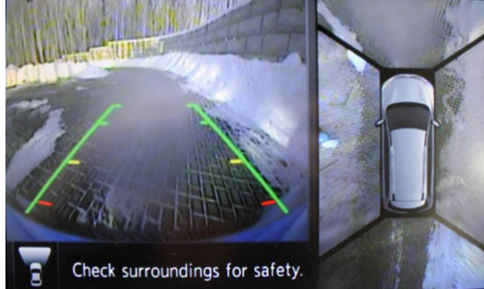
Fig. 1. Nissan Around view monitor system.
