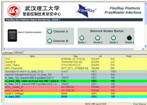
Fig. 9. The running interface of monitoring software of FlexRay bus platform.
