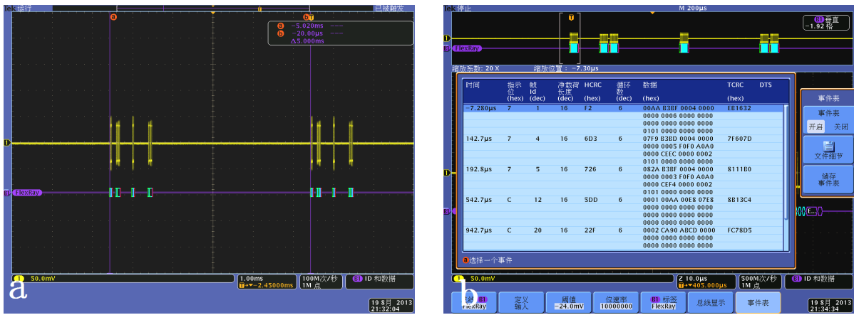
Fig. 6. The network period captured by MSO4104B.
