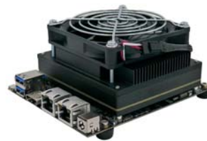
Fig. 22. Auvidia X230 carrier board with Orin AGX [22].
