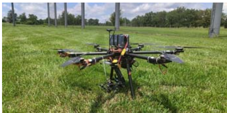
Fig. 20. The integrated Tarot T960 with camera payload and computing platform.
