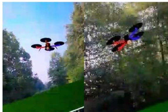
Fig. 8. ROS-Gazebo simulation: SITL flight in the urban flood Gazebo world with the YOLOv8 bounding box overlaid on the simulated camera feed and the lawnmower waypoint path active.
