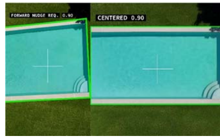
Fig. 5. Onboard target detection: YOLOv8 identifies the pool (simulated disaster zone), computes a heading-aware nudge to center over the target, and signals alignment (“Centered”).
