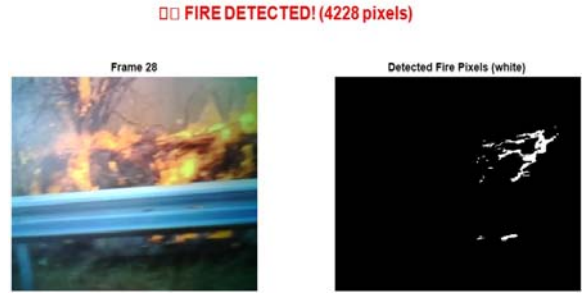
Fig. 4. Fire-region segmentation mask from the proposed hybrid model.
