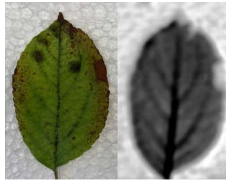
Fig. 16. Fresh leaf from an apple tree with some disorders and the corresponding terahertz image on the right.
