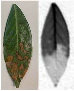
Fig. 13. Leaf in the drying process with terahertz image on the right.
