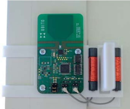
Fig. 10. Demonstrator including two Wiegand power sensors and the application circuit board.
