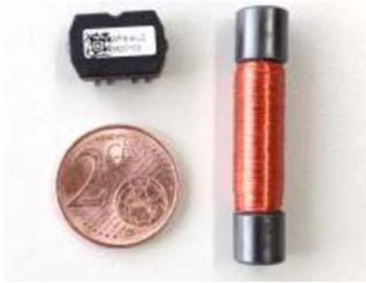
Fig. 5. High energy Wiegand sensor compared to standard WFS sensor.
