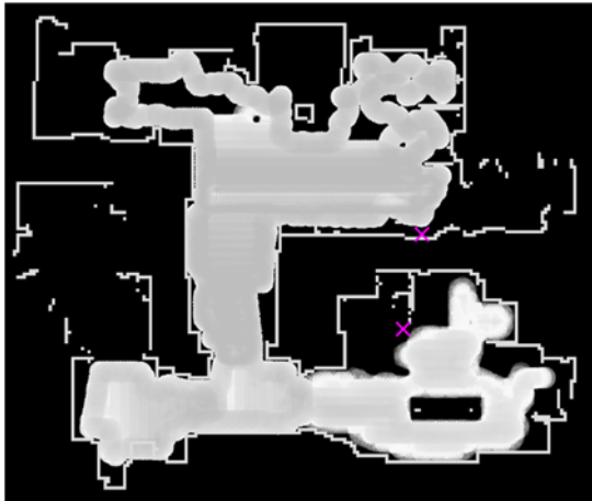
Fig. 7. Presence map, showing visited areas in white (except walls). Pink 'x's mark positions of obstacles that could not be removed as the robot did not visit the area.
