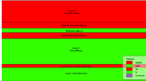
Fig. 1. Simulated \text{Ge}_{1-p}\text{Pb}_p/\text{Ge}_{1-x-y}\text{Si}_x\text{Pb}_y heterostructure.
