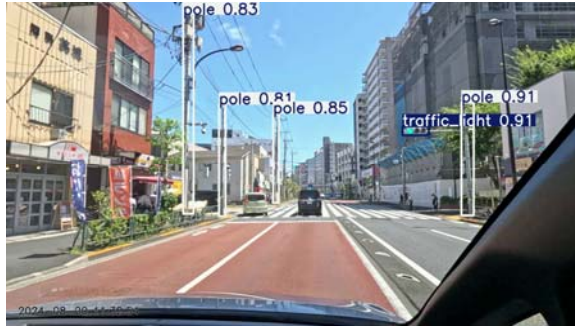
Fig. 8a. YOLO detected image of the start point of the evaluation course. The first trip at 11:32:54.
