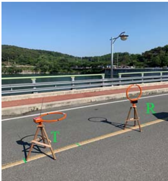
Fig. 1. Ground Penetrating Radar SDI K-5 on the dam at Nonsun, Republic of Korea. T is the radio wave transmitter, R is the receiver.
