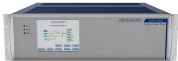
Fig. 1. High performance optically-pumped cesium beam clock OSA-3300. This clock fits in a standard 19'' rack, 133 mm high (3U) and is 450 mm deep. It weighs 23 kg and consumes 35 W at ambient temperature.
