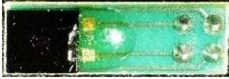
Fig. 1. Photograph of the Pd-doped graphene chemiresistor mounted on a carrier printed circuit board (PCB), used for gas-sensing response analysis.
