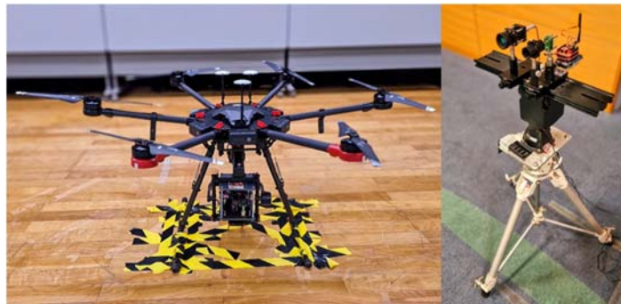
Fig. 2. (a) Drone with mounted Lasercom Module; (b) Ad-hoc optical receiving system.
