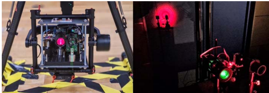
Fig. 4. (a) Lasercom module with downlink laser beam switched on (b) Footprint of the laser beam at the receiver.
