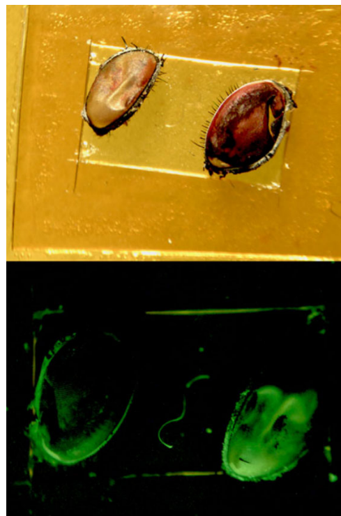
Fig. 2. Photographs of two blowfly corneas mounted on a glass slide, (top) before and (bottom) after being coated with Alq3. The top photograph was taken under normal illumination, but the bottom one was taken under shortwave-ultraviolet illumination.
