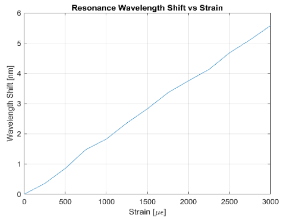
Fig. 6. Mode 6 resonance wavelength spectral shift vs adhesive associated stress.
