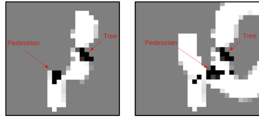
Fig. 5. Occupancy maps in two different moments. The pedestrian has another position and some cells of the previous position have been classified as trafficable.
