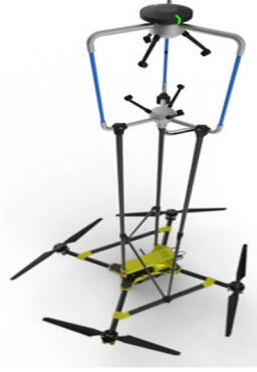
Fig. 1. Quadcopter with a deployed Ultrasonic-Anemometer [5]
