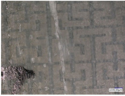
Fig 5. Microscopic image showcases the composite structure following the drop ball test, exposing the propagation of cracks within the composite material.
