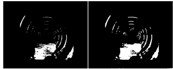
Fig. 5. Left, m_2 . Right, image with filled holes by the morphological filling operation.
