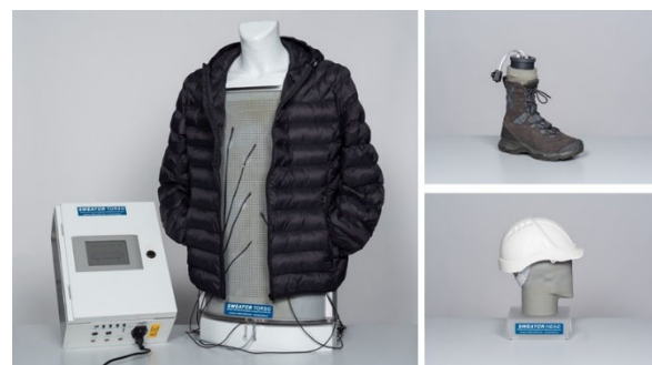
Fig. 6. SWEATOR torso with test jacket, SWEATOR foot and SWEATOR head with safety helmet.
