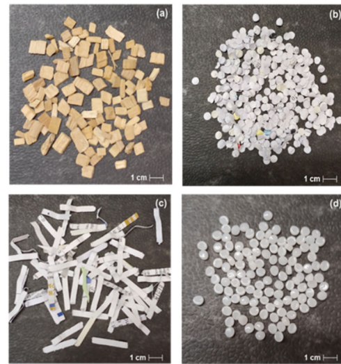
Fig. 2. Various RDF fractions applied in the experiments. (a) Wood chips. (b) Confetti. (c) Paper shreds. (d) PE granules. [10]
