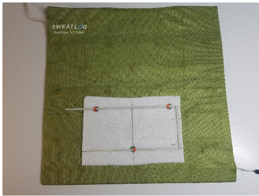
Fig. 4. SweatLog sensor array as sensor mat.
